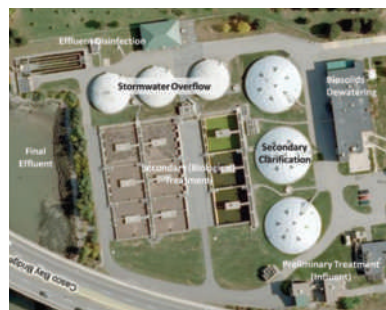
Figure 11.43 Your Neighborhood MSTP Communities use different components of wastewater treatment depending on their needs. This aerial view of a wastewater treatment plant in Portland, Maine shows primary and secondary treatment.
